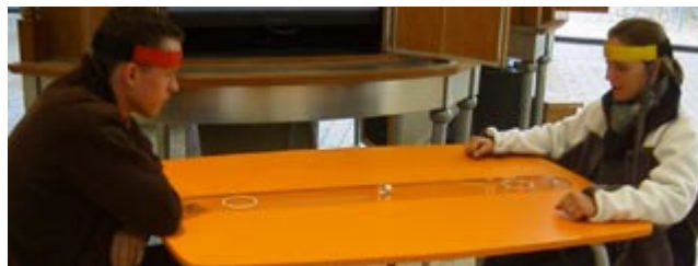
Fig. 2. Brainball: players' EEG signals control the movement of a physical ball on a table.
